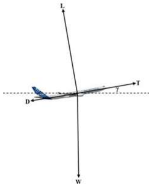
Figure 2. Forces acting on an aircraft using point-mass model.
